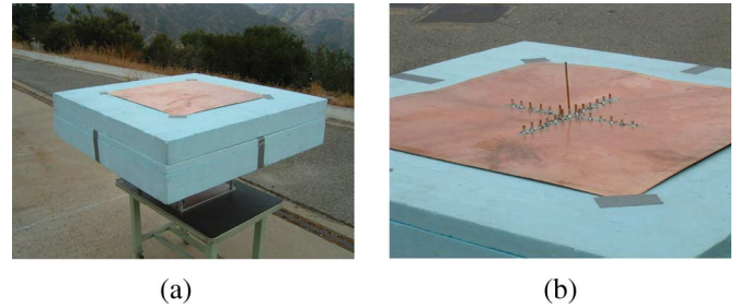
Fig. 4. (a) Photo of the whole antenna with top patch shown; (b) photo showing the bottom patch with the top patch removed.
